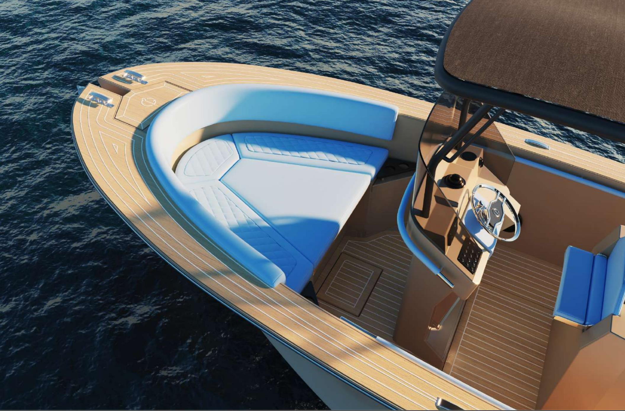
**Beneath the refined appearance of the Levanzo 25 "Lounge Deck" lies a heart of cutting-edge power and performance. The characteristic flared bow and hull lines allow this model to navigate rough seas, ensuring a dry deck for the crew and excellent stability. The navigation experience is further enhanced by the deep "V" hull with a 22° deadrise, providing impeccable agility and maneuverability.**
